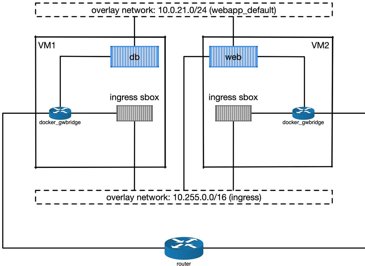
Fig. 8.3: An illustration of the Docker ingress network and routing mesh.
