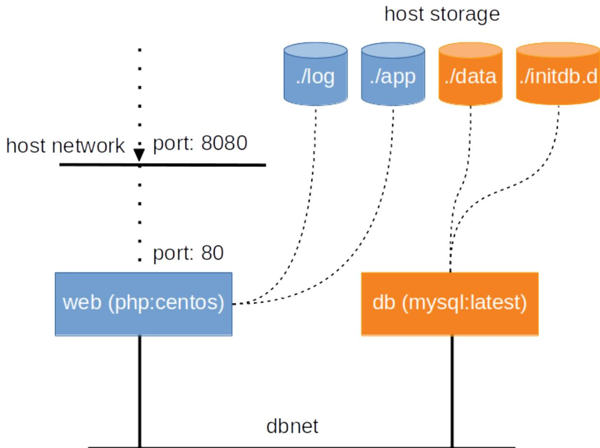
Fig. 7.1: an illustration of the service architecture implemented by the docker-compose file used in this tutorial.
