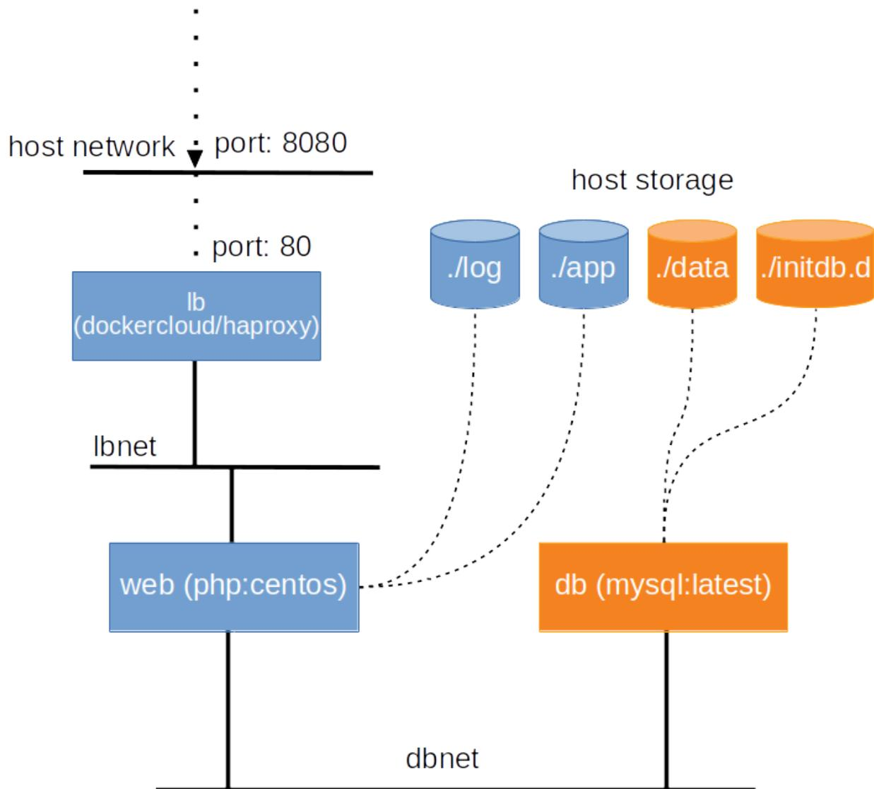
Fig. 7.2: an illustration of the service architecture with HAProxy as the loadbalancer.
